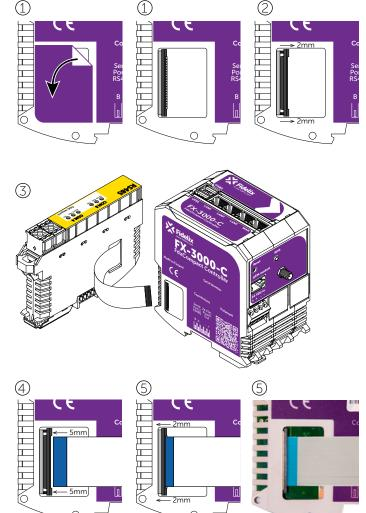
The connector is 22.5 mm wide (compared to 19 mm for the module itself), allowing for a small gap between the module and the controller.
