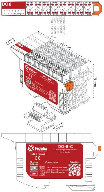
**Installation:** Tilt the module with the rounded corner towards the DIN-rail and then slide and click it onto the connector. As the connector is 22.5 mm wide, the small gap between modules allows for tidy and uncluttered cabling.
