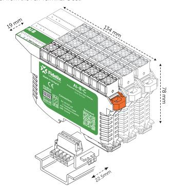
**Installation:** Tilt the module with the rounded corner towards the DIN-rail and then slide and click it onto the connector. As the connector is 22.5 mm wide, the small gap between modules allows for tidy and uncluttered cabling.
