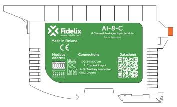
**LEDs:** The type of measurement will be shown on the module's label; per channel there are 2 LEDs, labelled "U" and "I" for voltage and current. If neither are lit, the AI-8-C module measures the resistance, which is also how the input is used as digital indication.
