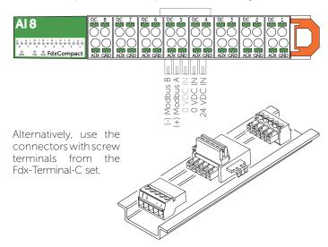
**Modbus address:** The address of the Al-8-C module can be set from 1 to 63 by changing the position of dip-switches 1-6. Each dip-switch represents a binary value, as indicated on the module (ST1...ST32).
