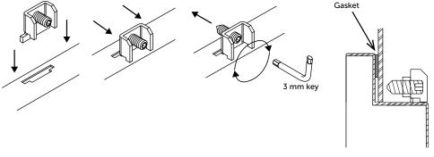
Alternatively, the FX-Vesamount set can be used to attach the display to a wall.
