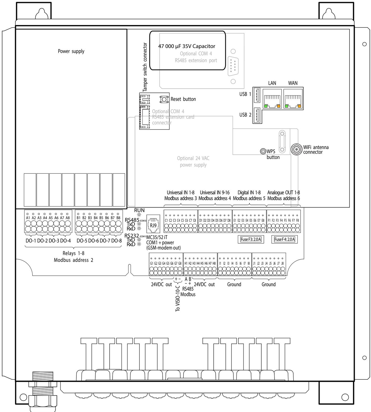
**Power supply:** The FX-SPIDER-40/10 controller comes with a standard European CEE 7/7 plug and is thus powered with 230 VAC. There is an adapter inside the encasing that powers all internal equipment, and also offers 24 VDC through connectors G1..G7 and H3..H8.
